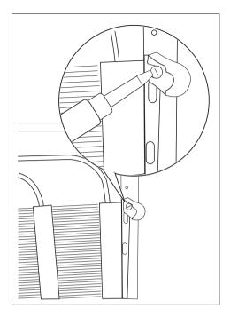
Slacken the screws and insert the spacer under the screw head, then retighten the screws.
